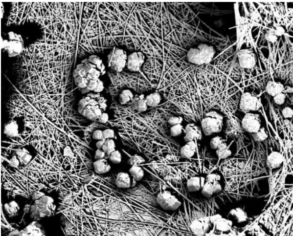
XYPEX TREATED CONCRETE (60% SLAG BLENDED CEMENT)
