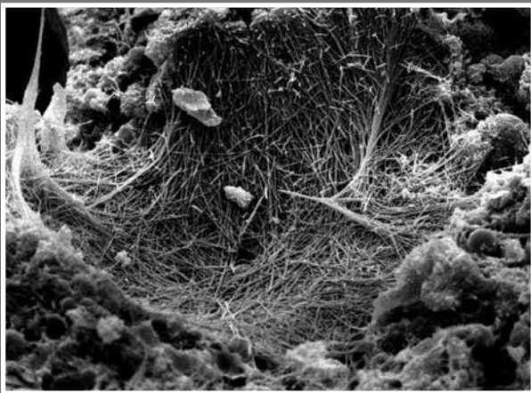
XYPEX TREATED CONCRETE
